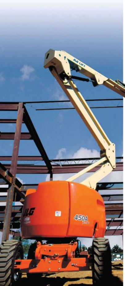
Jib-equipped models add 70 degrees of upward and 60 degrees of downward motion.
