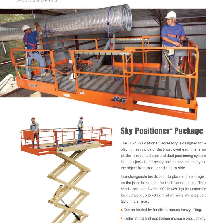
The JLG Sky Positioner® accessory is designed for workers placing heavy pipe or ductwork overhead. The removable, platform-mounted pipe and duct positioning system includes jacks to lift heavy objects and the ability to position
